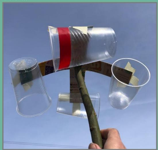
An anemometer is used to measure wind speed, but the children can make their own to compare the wind speeds at different places around the school.
